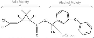
Figure 1: Typical structure of pyrethroids illustrated in Cypermethrin.<sup>24</sup>
